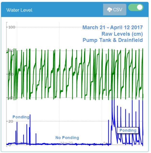
Significant variation in trench ponding levels has been observed. **Sometimes** levels approach the ground surface, while other times there is no ponding at all.
