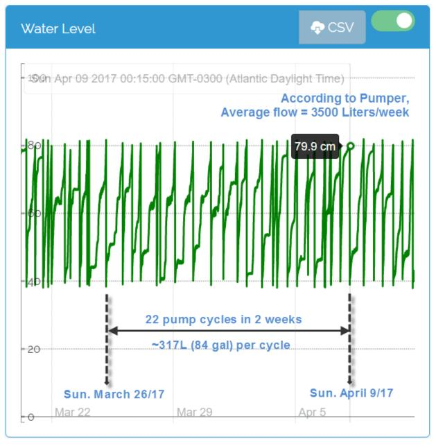
Septic Sitter data used to determine number of pump cycles in a 2 week period, and estimate the volume per pump cycle (dose)
